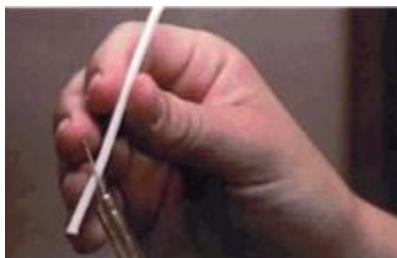
Slide the adjusting lever back down to draw the new wick into the lighter.
